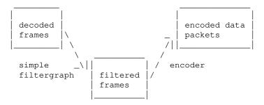
Simple filtergraphs are configured with the per-stream -filter option (with -vf and -af aliases for video and audio respectively). A simple filtergraph for video can look for example like this:
