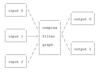
Complex filtergraphs are configured with the <code>-filter\_complex</code> option. Note that this option is global, since a complex filtergraph, by its nature, cannot be unambiguously associated with a single stream or file.
