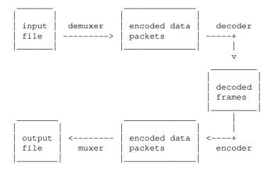
ffmpeg calls the libavformat library (containing demuxers) to read input files and get packets containing encoded data from them. When there are multiple input files, ffmpeg tries to keep them synchronized by tracking lowest timestamp on any active input stream.
